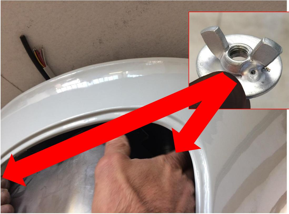
E) Use the 2 wing nuts to fasten definitely the shell to the structure.
