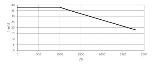
The above data are measured in connection with 2-4 DL16 lifting units and control box CBD4/CBD6S. The desk is driving upwards.
