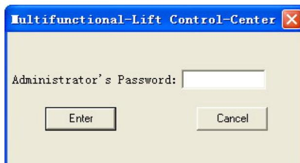
The user enter the correct administrator password, the software transfer to the administrator mode, the user can enter the grouping set up window to operate the window.
